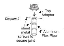
Pass the flex pipe down through the center of the chimney system, and center the adaptor on the top of the chimney pipe. Drill four 1/8" diameter holes through the adaptor and into the chimney top. Insure that you are in fact, drilling into the metal on the chimney. Twist-lock the Termination Cap (Part# 980 or 991) onto the Adaptor. (Diagram 3 and 4).
